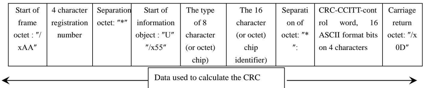
**Algorithm for calculating aCRC-CCITT-16bit control word**
