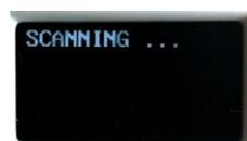
Very important : the PC can communicate with the reader only when the display of the reader is showing "SCAN".
