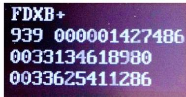
ISO FDXB tag compatible with the possibility to write additional data (+)
