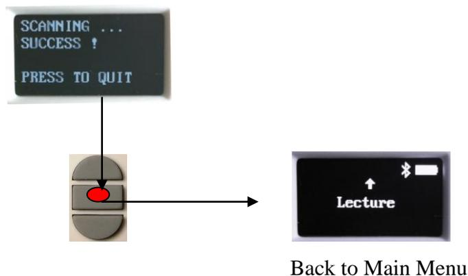
We recommend that you re-read the injected chip to verify that the data has been recorded, given that if the entry has been done correctly in the "chip" V8BT displays the following message:
