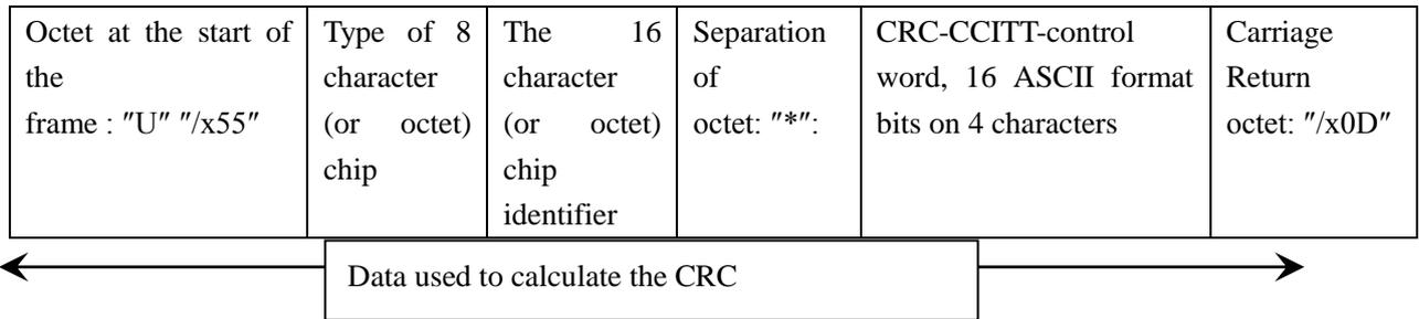
Tips: the developers of software associated with PetScan must use the head and separation characters to separate the information transmitted by PetScan, calculate a control word with the data received and compare it to the word transmitted by the PetScan to validate the information (see appendix for the CRC-CCITT-16 bit calculation algorithm)
