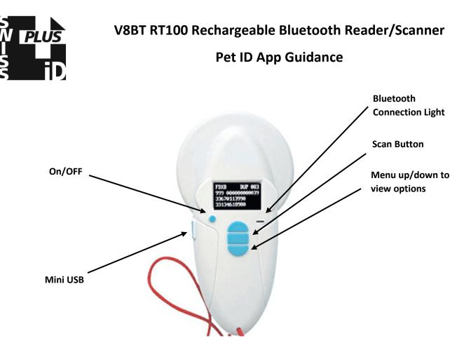
Guidance for using the Pet ID App function of the Realtrace V8BT RT100 Rechargeable Bluetooth Reader/Writer in conjunction with SwissPlus ID microchips.
