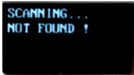
2 / you try to write a different chip than the one that was originally read,
